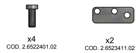
PLACING N°2 STOP AND SECURE THEM WITH THEIR SELF-THREADING SCREWS M5x16.
