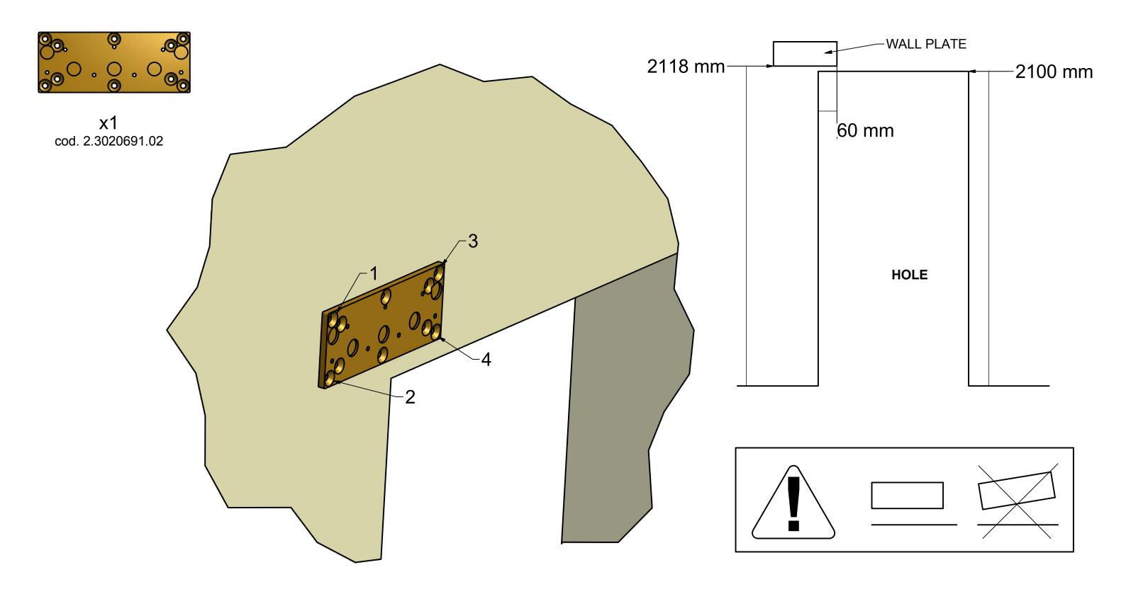
PLACE THE WALL PLATE, TAKING CARE THAT IS CORRECTLY ALIGNED, AND DRILL THE WALL, TO INSERT PLUGS Ø10 mm, THROUGH HOLE 1,2,3,4.
