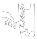
Press the fixing button while the safety handle button is pressed.
