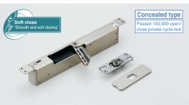
Unique door damper applicable to door weight up to 100 kg. Suitable for door weight 40~100 kg. Damper body is completely hidden when the door is closed.
